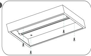
Install the fixture. Refer to previous page to find details on mounting holes.
