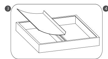
Gently push out the reflector from the holders and pull up one at a time, and remove both reflectors carefully.
