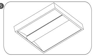
Reinstall in order of two reflectors, module plate, then diffuser at last.
