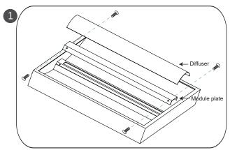
Remove diffuser carefully, unscrew 4 screws to remove module plate.
